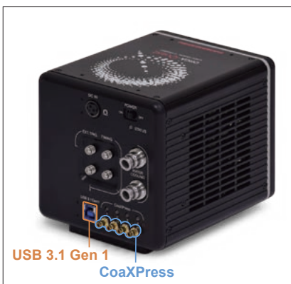
Fig. 3-2. CoaXPress and USB 3.1 Gen 1
